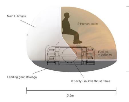
Eight, 3G thrusters give multiple redundancy, allowing up to four to fail.
